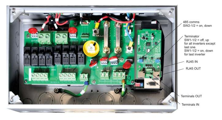
Fig 3 K135 Gateway to inverters connections
